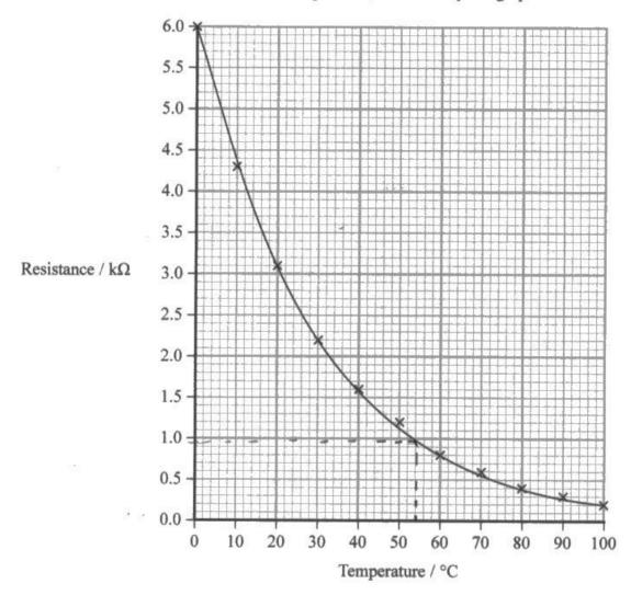
(a) Determine the milliammeter reading when the temperature of the thermistor is 54°C.
