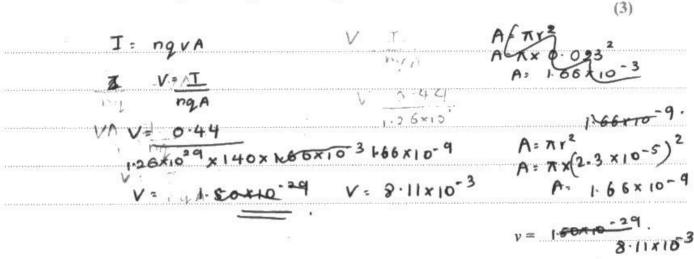
(ii) When the potential difference across the tungsten filament is 140 V the current in the filament is 0.44A.
