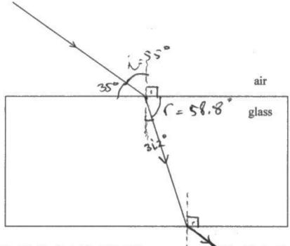
(a) Complete the diagram to show the path of the ray as it enters the block. Use the space below for any calculations.
