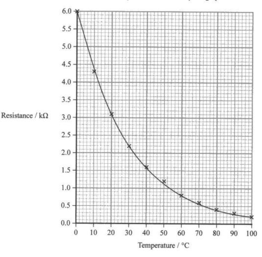
(a) Determine the milliammeter reading when the temperature of the thermistor is 54°C.
